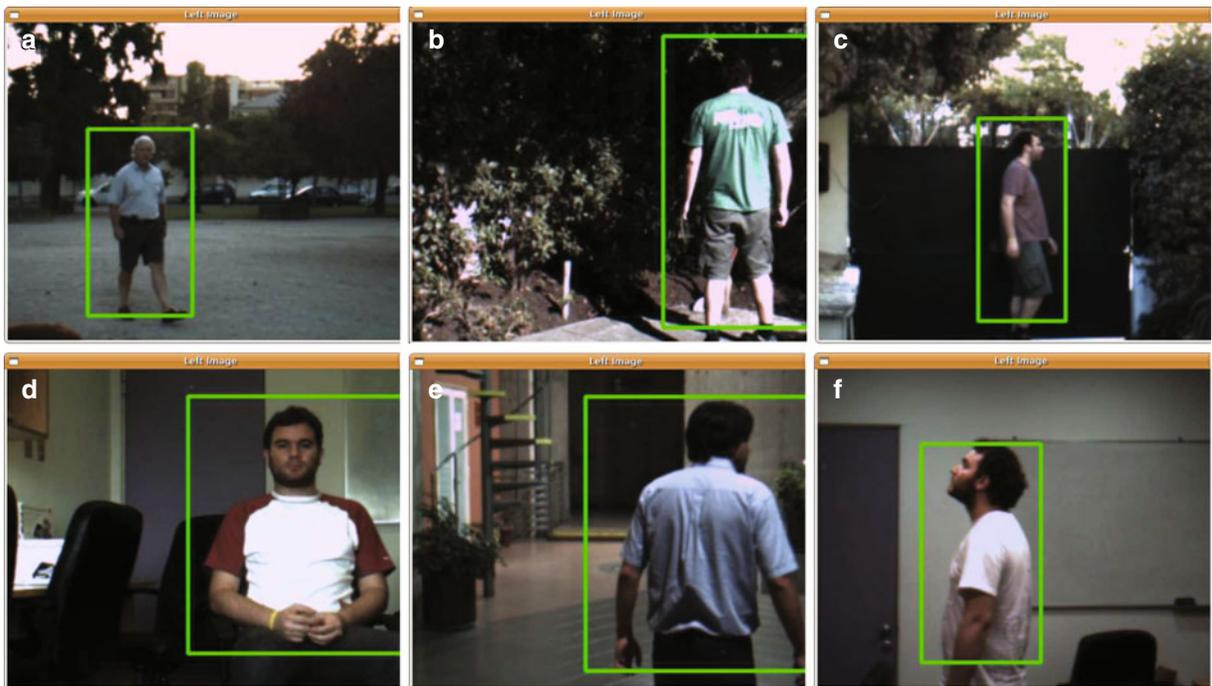
**Fig. 8** Figures a–f present results of our human detection system able to detect people under different poses. The system uses a new fast feature descriptor based on visual
